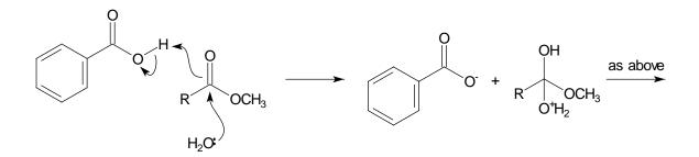
The equation for the observed rate constant for this type of reaction includes a term for each undissociated acid (HA) in the reaction.
