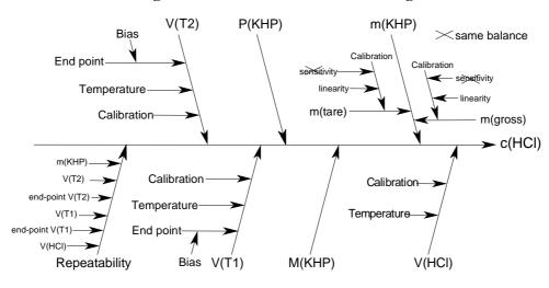
Figure A3.5: Final cause and effect diagram
