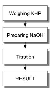
Figure A2.1: Standardising NaOH
