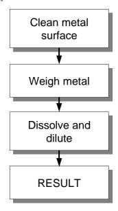
Figure A1. 1: Preparation of cadmium standard
