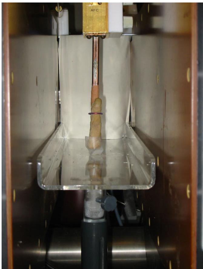
**Figure 1.** Picture of a human finger inserted into the surface-coil resonator in the gap between the electromagnet pole shoes of the L-band spectrometer.
