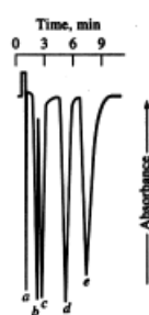
Figure 28-24 Indirect photometric detection of several anions by elution. Eluent: 10^{-3} M disodium phthalate, 10^{-3} M boric acid, pH 10. Flow rate: 5 mL/min. Sample volume: 0.02 mL. UV detector. Sample ions: (a) 18- \mu g carbonate; (b) 1.4- \mu g chloride; (c) 3.8- \mu g phosphate; (d) 5- \mu g azide; (e) 10- \mu g nitrate. (Reprinted with permission from H. Small, Anal. Chem., 1985, 55, 240A. Copyright 1983 American Chemical Society.)
