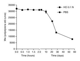
Fig. 3. Stability study of nanoparticles consisting of 1:1 (w/w) PEG-b-PLA: PLGA, produced by double emulsion, evaluated by measuring polymer molecular weights by GPC. Nanoparticles were incubated for 56 days in PBS at 37 °C or incubated for 2 h in 0.1 M HCl at 37 °C (simulated gastric fluid) (n=2).
