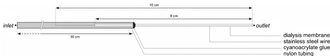
Fig. 2 – Linear DMD probe.
