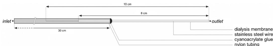
Fig. 2 – Linear DMD probe.
