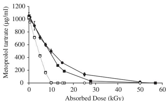
Fig. 5. Metoprolol tartrate concentration in  $\mu\text{g ml}^{-1}$  as a function of absorbed dose in kGy, for irradiations of metoprolol tartrate ( $1\text{ mg ml}^{-1}$ ) solutions, saturated in nitrogen. E-beam irradiation (—■—), gamma irradiation (—●—), e-beam simulation (---□---) and gamma simulation (---○---).
