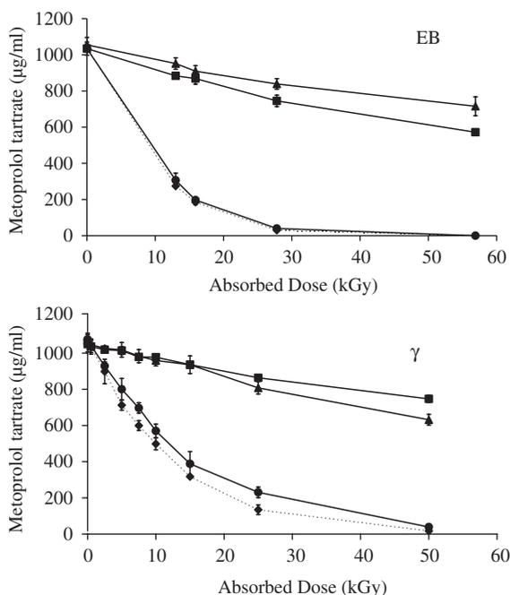
Fig. 6. Metoprolol tartrate concentration in  $\mu\text{g ml}^{-1}$  as a function of absorbed dose in kGy for e-beam (EB) and gamma ( $\gamma$ ) irradiations of metoprolol tartrate ( $1 \text{ mg ml}^{-1}$ ) solutions, saturated in nitrogen and containing the following excipients: 0.9% NaCl ( $\bullet$ ), 2% 1,2-propanediol ( $\blacktriangle$ ), 5% mannitol ( $\blacksquare$ ), no excipient ( $\blacklozenge$ ).
