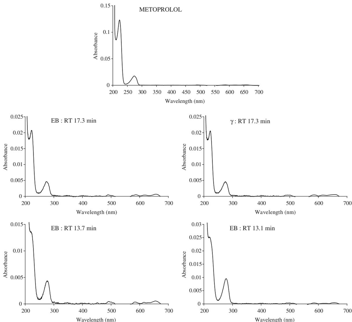
Fig. 3. DAD spectra of metoprolol with retention time 20 min and main radiolytic products with retention times 17.3, 13.7 and 13.1 min. EB: electron-beam irradiation of 12.8 kGy.  $\gamma$ : gamma irradiation of 10 kGy. Metoprolol tartrate ( $1 \text{ mg ml}^{-1}$ ) solutions, saturated in nitrogen.
