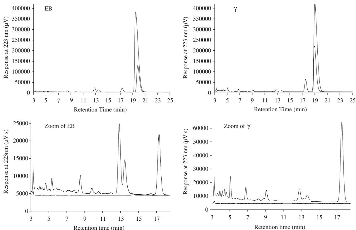
Fig. 2. Overlay of non-irradiated and irradiated chromatograms, at 223 nm, of metoprolol tartrate ( $1 \text{ mg ml}^{-1}$ ) solutions, saturated in nitrogen. Zoom on radiolytic products prior to metoprolol peak. EB: e-beam irradiation of 12.8 kGy.  $\gamma$ : gamma irradiation of 10 kGy.
