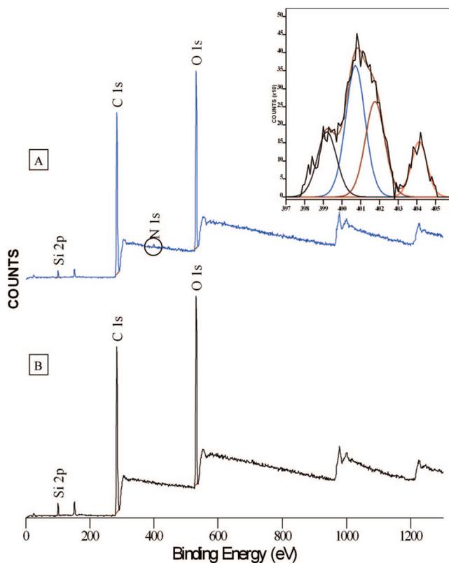
**Figure 2.** (A) General XPS survey scan of PCL-PEG-g-GRGDS-1; (B) general XPS survey scan of PCL-PEG-AP1; inserted spectra shows the nitrogen signal at high resolution.
