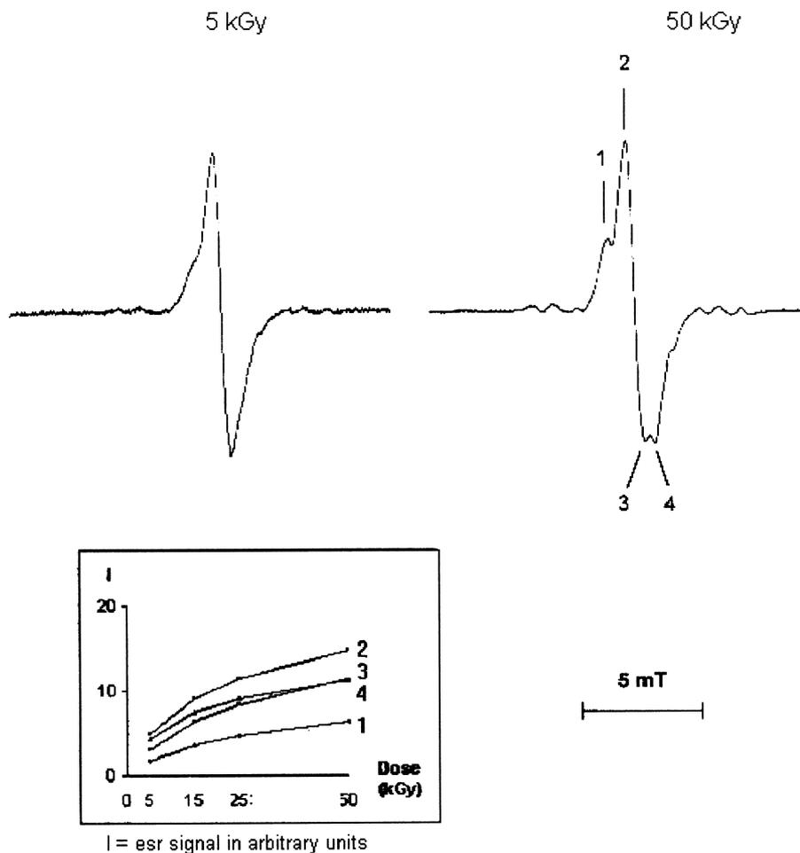
Fig. 4. Influence of irradiation dose on AAT ESR spectra. The lines numbers of the curves put in the scroll correspond to the ones of the right spectrum. The doses are of 5 and 50 kGy respectively; without irradiation, ESR spectrum is not registered. Relative ESR area are given for each peak as a function of dose.
