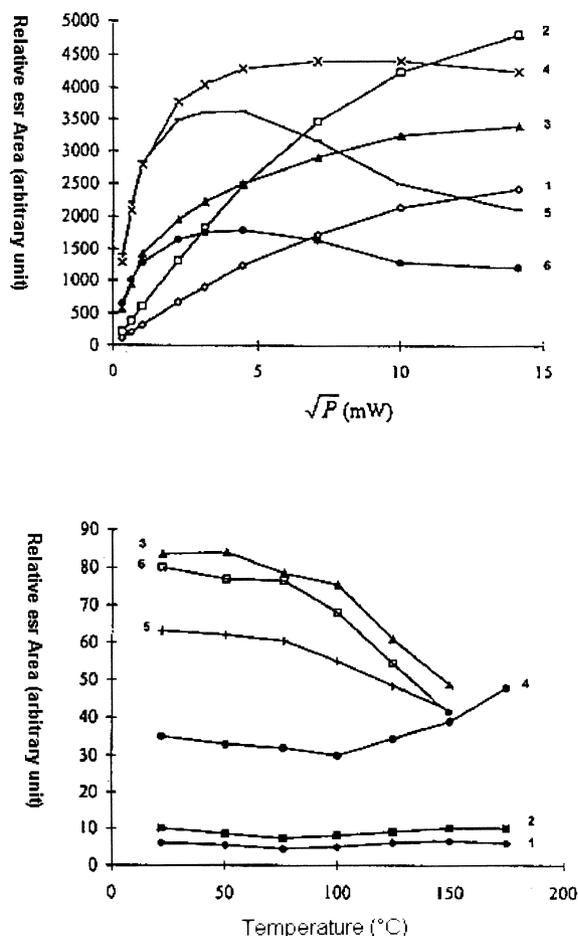
Fig. 3. Influence of microwave power (top) and of recording temperature (bottom) on relative intensities of ESR spectra (arbitrary units) of irradiated (25 kGy) AAA (the lines numbers are defined on the AAA spectrum of Fig. 2). We use a microwave power of 400  $\mu$ W to avoid saturation.
