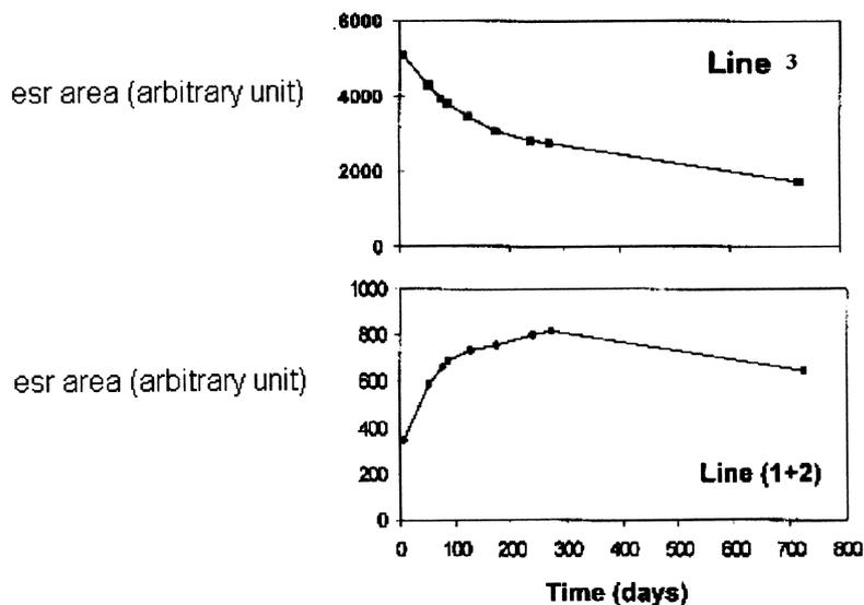
Fig. 5. Influence of storage time at room temperature on two lines of the irradiated AAA ESR spectrum (the different lines are defined on Fig. 2) at 25 kGy.
